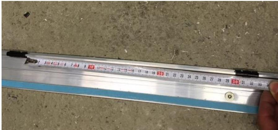
Check if the clip is correct positioned to avoid assembly issues in further steps!
